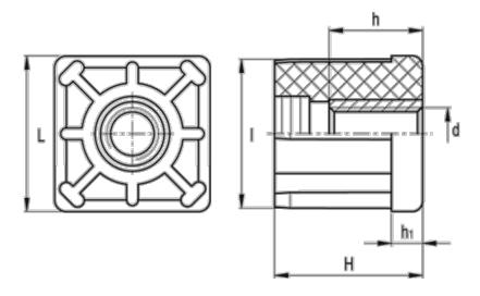
$\begin{array}{lll} d & = M20 \\ h & = 20 \\ H & = 45 \\ h1 & = 10 \\ Internal tube size = 45.0 \\ I & = 45.0 \\ L & = 50 \\ \end{array}$
